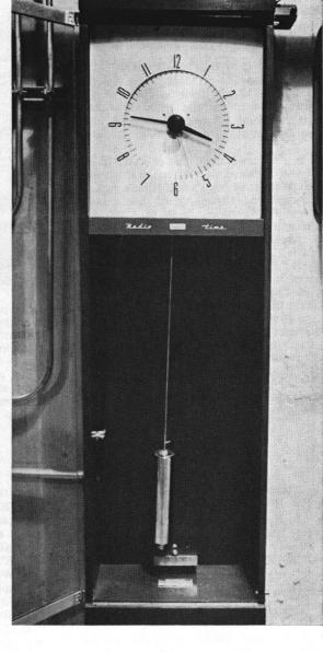
PLASMA FACILITY uses this Dwell Timer to control duration of plasma tests. Bill Jacklin (7335) calibrates the timer. Exposure of test items in the facility can be controlled to intervals accurate within half a second.
